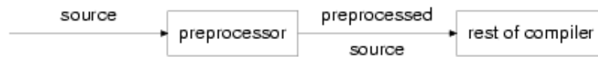
Figure 7.1: Diagram showing source code passing through a preprocessor to become 'preprocessed source', which is then fed into the rest of the compiler.
